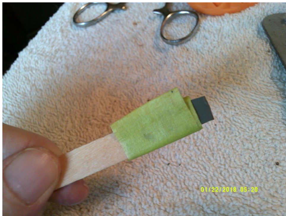
Stick with end pointed, and 2000 grit taped on.
