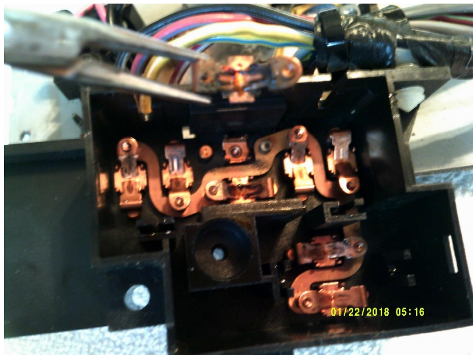
Before cleaning, using hemostat to remove.
