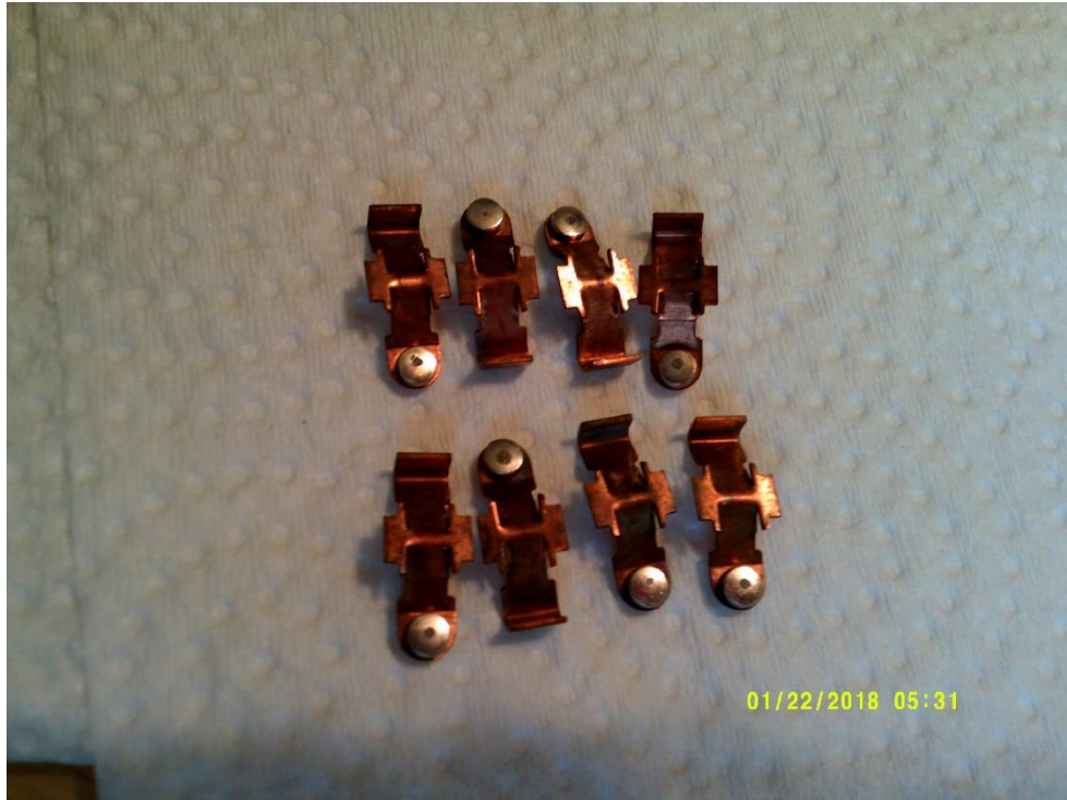
8 contact pieces removed and cleaned.
