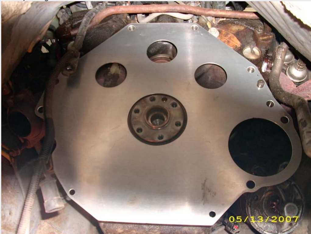
Flywheel, reuse your flex plate bolts, stick some blue threadlocker on, and then torque to 90 ft/lbs
