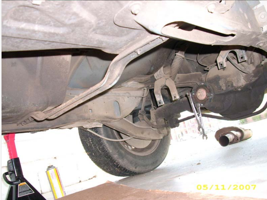
After draining the trans, unbolting the torque converter nuts, bellhousings bolts, and trans cooler lines drop the DOA. Using a transmission jack makes this a lot easier.
